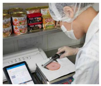
Ms Yap Jia Huan, using the e-datalogger to record the inspection results of the finished product measurement
